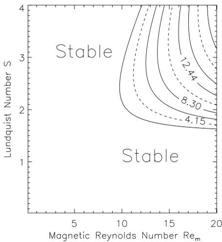
FIG. 2. MRI linear growth rates ( $\gamma$  s $^{-1}$ ) as a function of magnetic Reynolds number  $Re_m$  and Lundquist number  $S$  with dimensions as in Table I:  $r_1 = 7.1$  cm,  $r_2 = 20.3$  cm, and  $h = 27.9$  cm and  $\mu = \Omega_2/\Omega_1 = 0.13325$ . The system is MRI stable if  $Re_m \leq 10$  regardless of  $S$ .
