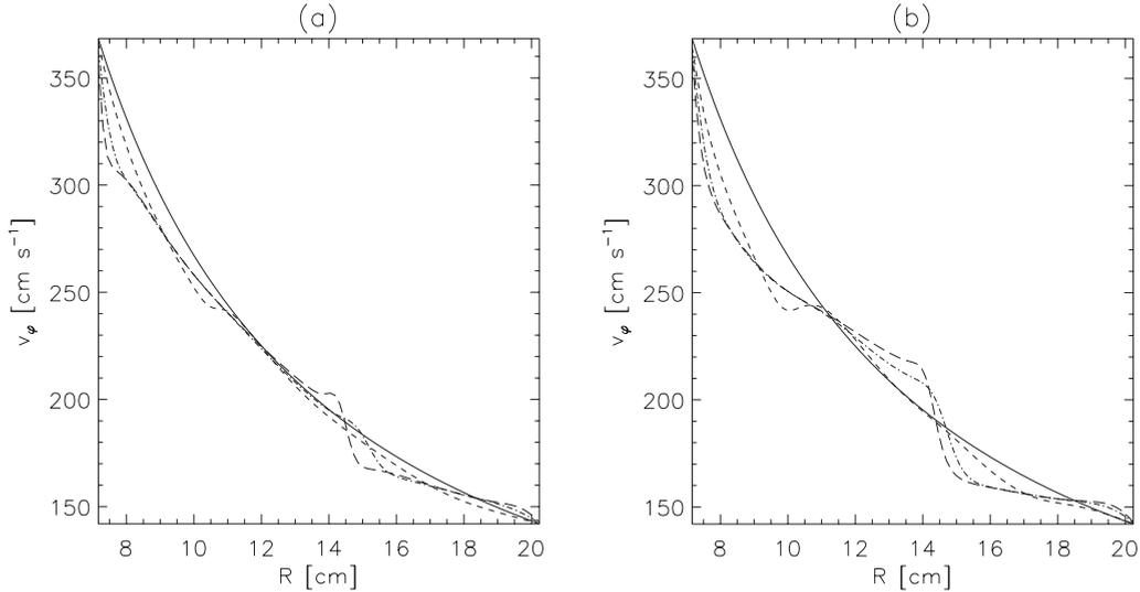
FIG. 9. Azimuthal velocity  $v_\phi$   $\text{cm s}^{-1}$  versus radius  $r$  at different heights with  $\text{Re}_m=2.5$ ,  $\text{Re}=6400$ , and the endcaps divided into two rings at  $r_d=(r_1+r_2)/2=13.7$  cm. Parameters as in Table I. Solid line, ideal Couette state; long dashes,  $z=1.33$  cm (relative to the bottom endcap); dash dot,  $z=2.79$  cm; short dashes,  $z=13.95$  cm. (a)  $\Lambda=0.38$ ; (b)  $\Lambda=1.5$ .
