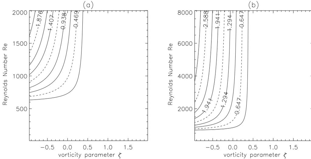
FIG. 12. MRI linear growth rates ( $\gamma \text{ s}^{-1}$ ) as a function of Reynolds number  $Re$  and vorticity parameter  $\zeta$  at the junction between rings,  $r_d=(r_1+r_2)/2$  with  $\Lambda=1.5$ . Parameters as in Table I. (a) the vertical mode number  $n=0.25$ ; (b)  $n=1$ .
