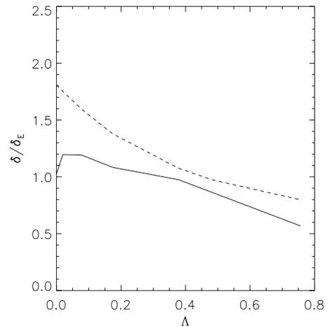
FIG. 4. The thickness of the Ekman layer  $\delta$  versus Elsasser number  $\Lambda$  for  $Re = 6400$ ,  $Re_m = 2.5$ . Parameters as in Table I. The data are measured at  $r = (r_1 + r_2)/2 = 13.7$  cm. The dashed line is from the linear analysis [Eq. (11)]. The solid line is obtained from modified ZEUS-2D simulations.
