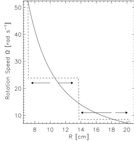
FIG. 8. Two independently rotating rings generate eight cells. Solid line, ideal Couette state; dashed line, rotation profile at the endcaps. Arrows indicate the radial flow directions near the endcaps.
