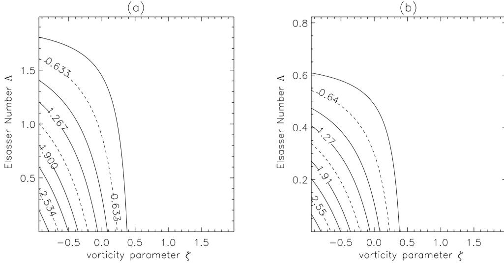
FIG. 11. Growth rates ( $\gamma$  s $^{-1}$ ) predicted by Eq. (13) as a function of Elsasser number  $\Lambda$  and vorticity parameter  $\zeta$  at the junction of rings,  $r_d=(r_1+r_2)/2$  with  $\text{Re}=6400$ . Parameters as in Table I. (a) the vertical mode number  $n=1$ ; (b)  $n=2$ .
