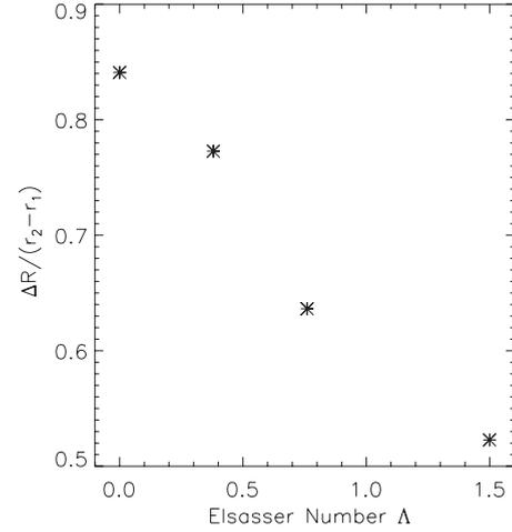
FIG. 6.  $\Delta R/(r_2 - r_1)$  vs  $\Lambda$ .  $\Delta R$  is the radial width of the dynamically active region.  $\text{Re}_m = 2.5$ ,  $\text{Re} = 6400$  with end plates corotating with outer cylinder. Parameters as in Table I. Note that in the simulations the magnetic diffusivity  $\eta$  is fixed to  $\eta \sim 2000 \text{ cm}^2 \text{ s}^{-1}$ , however, the imposed axial magnetic field  $B_{z0}$  is varied.
