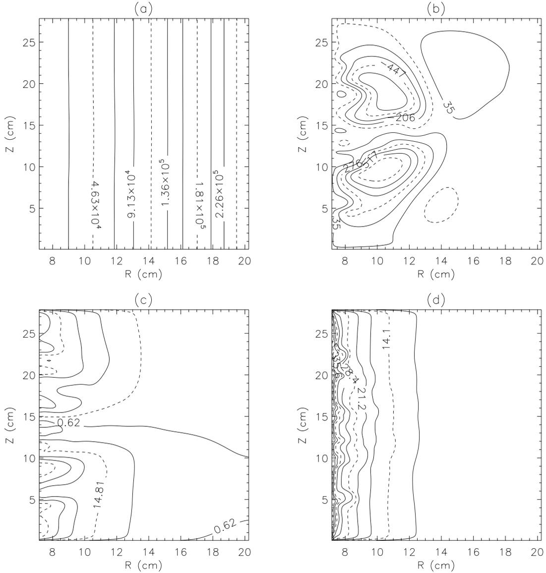
FIG. 5. Contour plots of final-state velocities and fields with uniformly rotating endcaps.  $Re=6400$ ,  $Re_m=2.5$  with  $B_{z0}=1500$  G ( $\Lambda=1.09$ ). Parameters as in Table I. (a) Poloidal flux function  $\Psi$  ( $G\text{ cm}^2$ ) (b) Poloidal stream function  $\Phi$  ( $\text{cm}^2\text{ s}^{-1}$ ) (c) toroidal field  $B_\phi$  (G) (d) angular velocity  $\Omega \equiv r^{-1}V_\phi$  ( $\text{rad s}^{-1}$ ).
