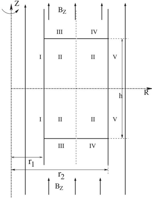
FIG. 1. Computational domain for studies of magnetic Ekman layer. Region (I) Perfect conducting inner cylinder, angular velocity  $\Omega_1$ , infinitely long. (II) Liquid metal. (III) Perfectly insulating inner ring  $\Omega_3$  extending to infinity. (IV) Perfectly insulating outer ring  $\Omega_4$  extending to infinity. (V) Perfectly conducting outer cylinder  $\Omega_2$  infinitely long. Thin dash line: the midplane.  $B_z$  is the initial background vertical uniform magnetic field.
